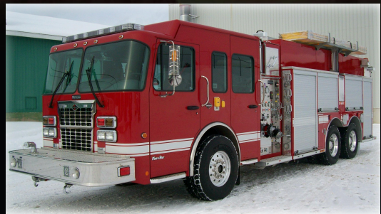
Our thanks to La Durantaye Fire Department, QC for choosing METALFAB to manufacture their new Pumper/Tanker: 2009 Spartan MetroStar, 4 Door Chassis • Hale QMAX 1250 IGPM • 2500 Imp. Gal. Ultra Tank • Extruded Aluminum Body
