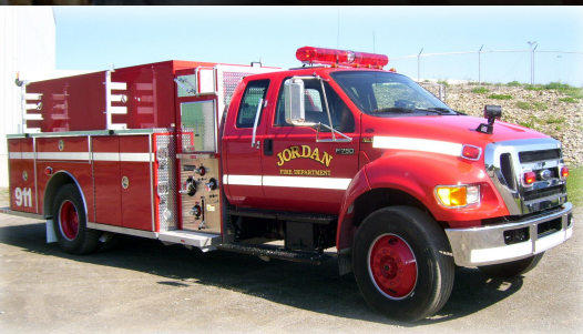
Our thanks to the Jordan Falls Fire Department, NS for choosing METALFAB to manufacture their new Tanker: 2008 Ford F-750, Extended Cab • Hale AP PTO 420 IGPM • 1000 Imp. Gal. Ultra Tank • Extruded Aluminum Body
